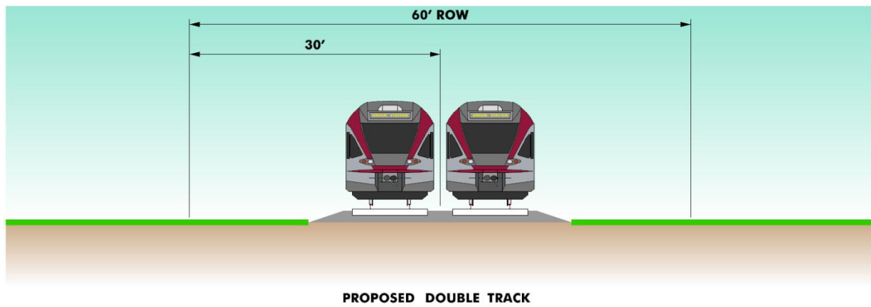
Figure 6: Regional Rail Typical Section on Common Segment – 2nd and Holmes Proposed Conditions
