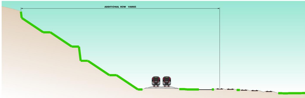
Figure 5: Regional Rail Typical Section on Common Segment (East of Chestnut Avenue) Kessler Park Proposed Excavation
